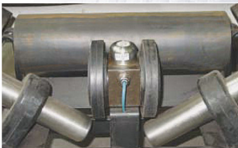
Belt track monitoring with the proximity switch iNA14
